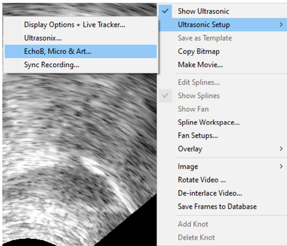
AAA has access to 4GB of memory as it is 32-bit code. It is not recommended to allocate more than half of that memory to ultrasonic and video data recording because other Windows programs may need it.
