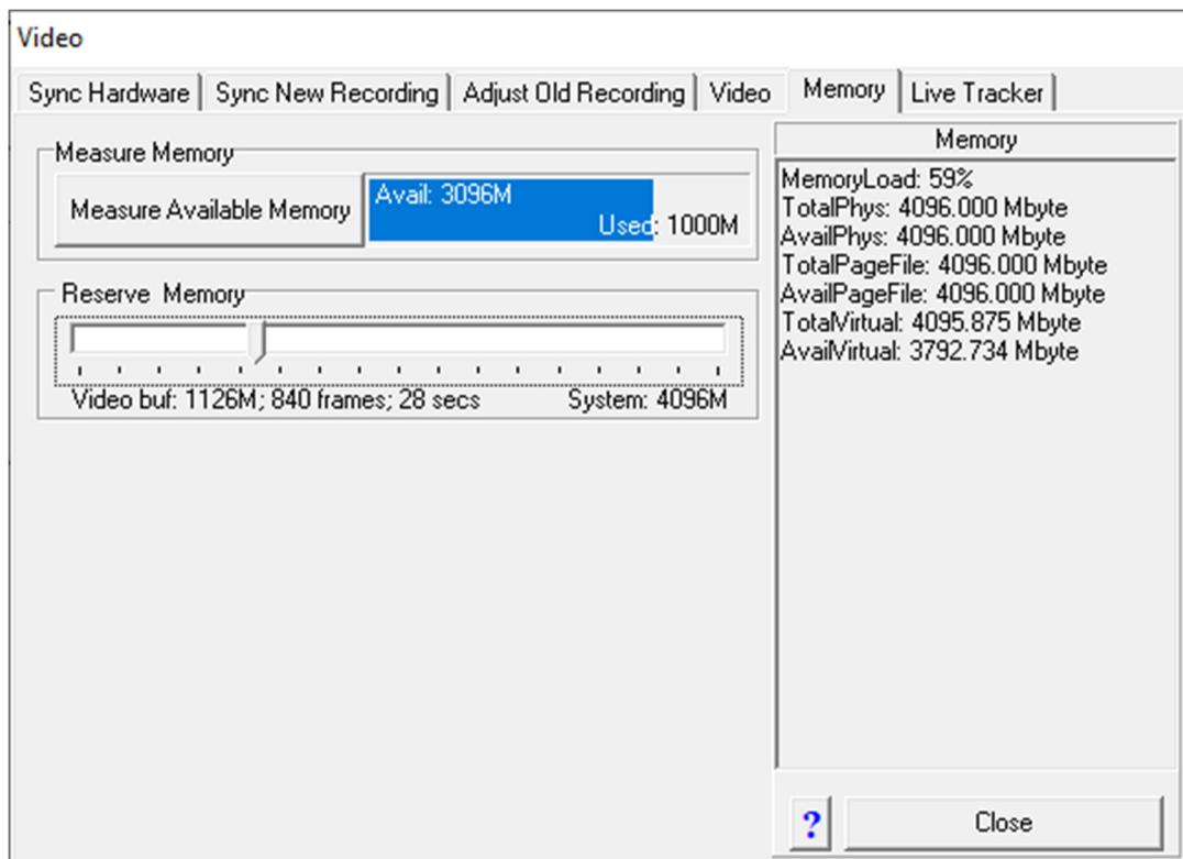
To record 2 minutes of greyscale video and ultrasonic data requires about 1.7Gb memory to be allocated (2 minutes of uncompressed 22kHz stereo audio is about 10Mb).
