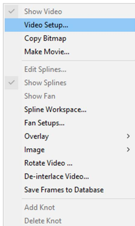
If you have a camera connected showing a live video signal then the estimated time in the memory dialog will be accurate. The time in the dialog below is not accurate. It is recommended that video is always recorded in greyscale as colour require 3x the memory of greyscale. As a rough guide, the 1126Mb allocated below should equate to about 2 minutes
