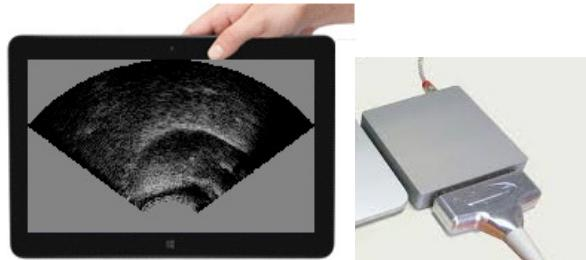
Radius 20mm; Frequency 2-4MHz; Max FOV 101.2°
